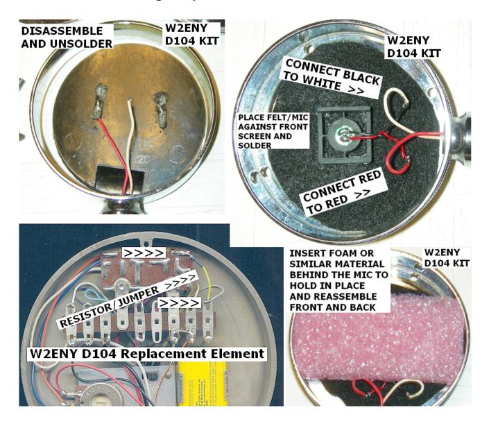
This is an FET electret element, you will need to add the supplied Resistor/Jumper in your T-UG8 Base to pass DC to the element.
