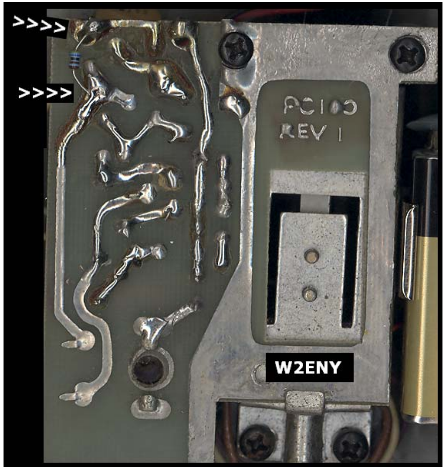
Bottom view showing the circuit board and the resistor's placement
