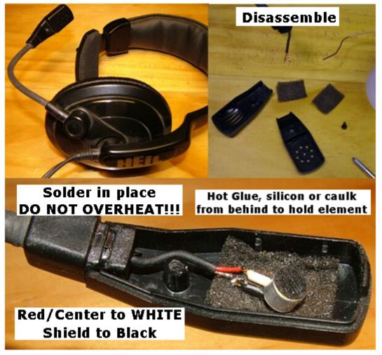
This is an FET amplified electret element, you will have to mod your Heil adapter cable to pass DC to power the element.
